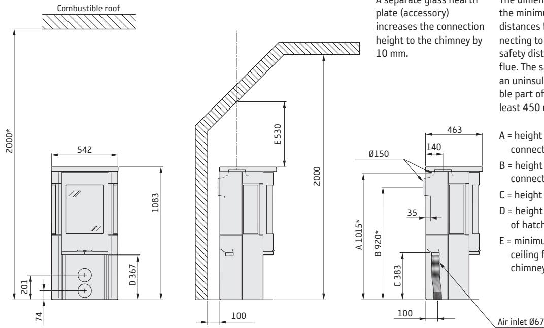
A separate glass hearth plate (accessory) increases the connection height to the chimney by 10 mm.
